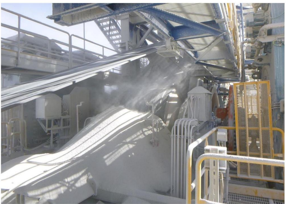
Headpulley is "grinding" more ore.
