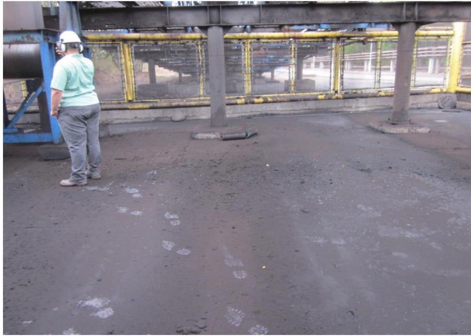
Massive contamination of CarryBack
