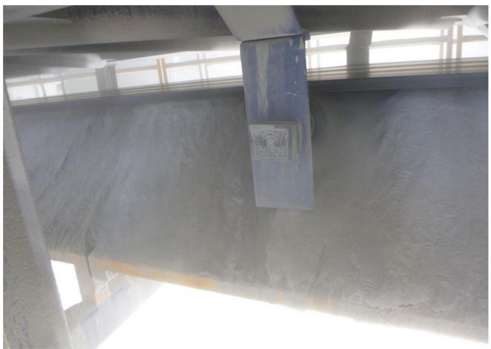
The return cable moves over Carryback, not on pulleys.
